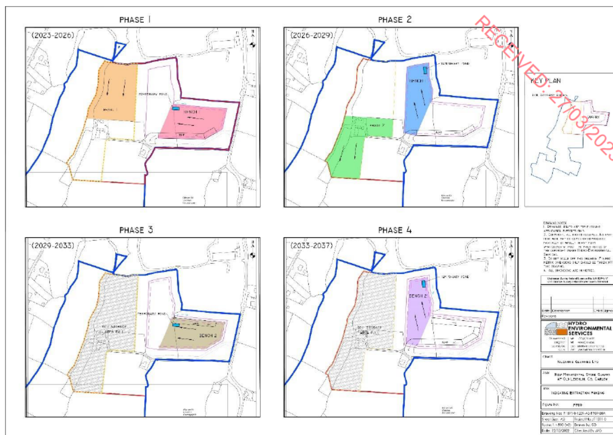
Figure 10-23: Indicative Extraction Phasing. Source: Hydro Environmental Services
